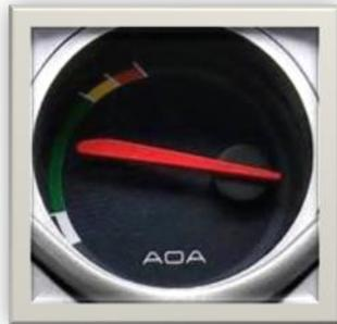
An AOA indicator can help when used in conjunction with airspeed and existing stall warning systems, when available. It can be used to get the pilot’s attention (via audio and/or low cost stick shakers) even if the pilot is not looking at it. This focuses the pilot’s attention on where it needs to be to avoid the stall.
